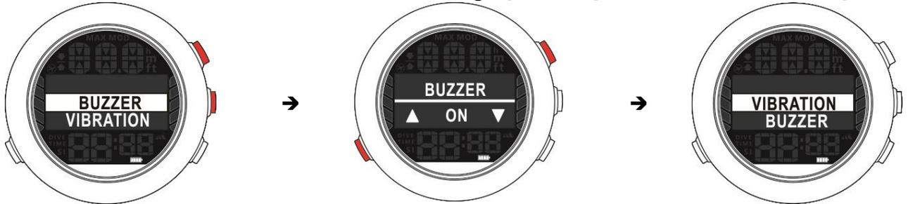
4. Select : [Button A] Switch "BUZZER" and "VIBRATION"
